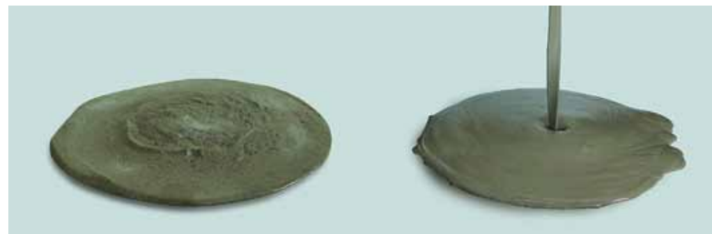
Beton s superplastifikatorjem Concrete with superplasticizer
