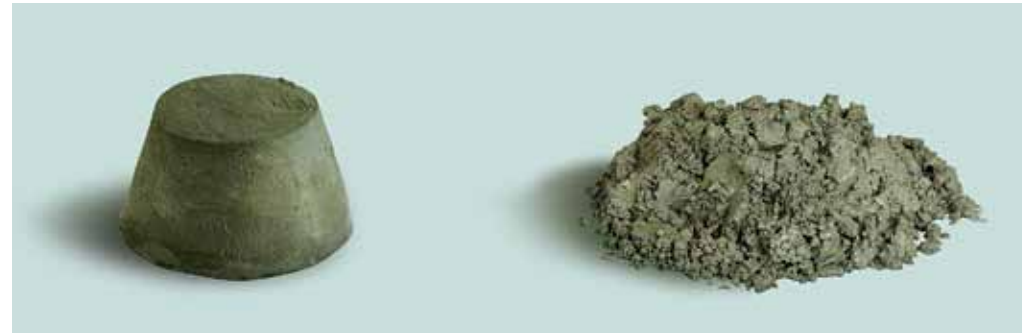
Beton brez superplastifikatorja Concrete without superplasticizer
